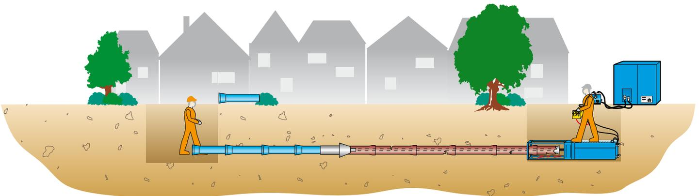
Push-pull technique/auxiliary tube technique
